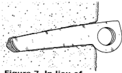
Figure 7. In lieu of glue-ins, a 1/2-inch angle piton hammered into a 3/8-inch hole is the most common soft-rock anchor.
