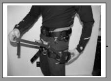
Thread buckle and attached strap from one side of Batten Seat through the triangular slot in the plate of the suspension assembly of Ergovation<sup>®</sup> saddle / sit harness as pictured above.
