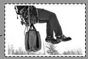
**Note**: Loops on exterior of batten seat are designed to store gear and suspend items like rope and rope bags while aloft. Items must not exceed 33 lbs. (15Kg).
