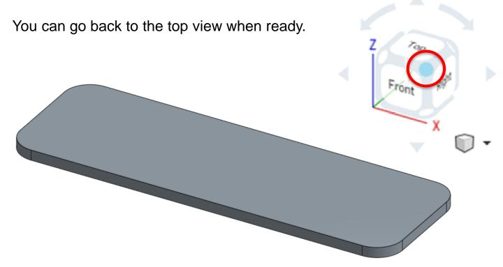
Let's make a new sketch for the hole. Holes have a special 3D button that puts a hole anywhere you have a sketch point.
