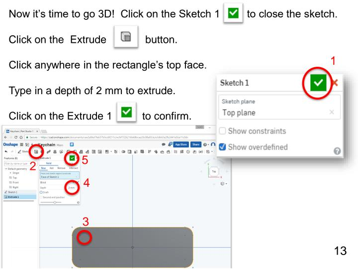
You now have a 3D part. To look around, use the cube in the top right corner to navigate around. Clicking on the corners of the cube gives you an **isometric** 3D view.
