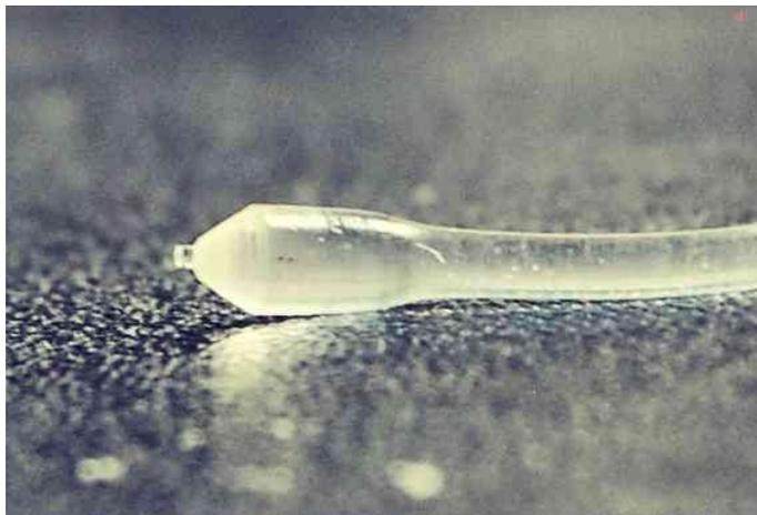
**NOTE: Every time you change filament on your 3D printer, remove the filament with the nozzle at around 100°C. This method usually removes all the old color of filament from the hot end, so when you begin printing again, the new color will begin printing immediately.**
