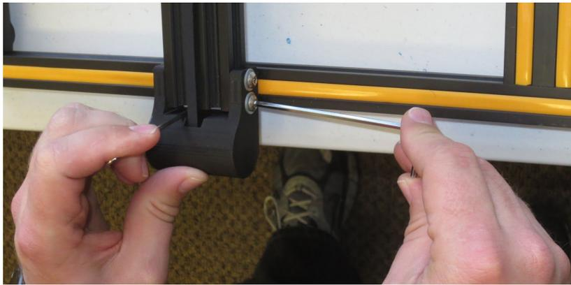
5. Check the tension of the belt driving the X-axis (on the gantry). The belt should be taut, with no slack or slop.
