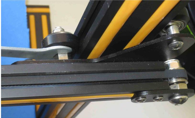
3. Adjust the tension of the nozzle assembly on the X-axis on the gantry frame.
