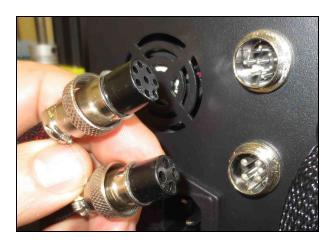
c. Connect the motor and limit switch cables.
