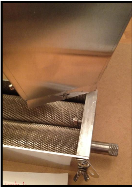
Figure 3: Alignment of hopper and roller base
