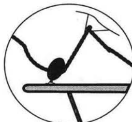
H-18SX H-21SE Rivet eye strap to outboard and rear of wing tube. Shackle block to eye strap. Twist on spring as though putting key on key ring. Spring holds block in upright position.
