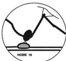
H-18 Rivet eye strap to outboard end of rear crossbar. Shackle block to eye strap. Twist on spring as though putting key on key ring. Spring holds block in upright position.
