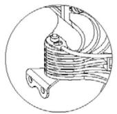
This new design has a simplified and more intuitive function: to raise the rudder, raise the tiller; to lower the rudder, lower the tiller. The rudder automatically locks into either position and is held by spring-loaded detents. The rudder will kick-up if beached or if an obstruction is hit.
