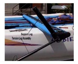
Install the tension leg assembly (the telescoping tube assembly) and the support leg (larger 2" tube) into the end cap casting as shown using the 3/8x3.5" bolt. Put some supplied Locktite on the threads.
