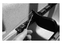
3. You want to adjust the amount of pull on each line so the rudder is straight. With the rudder straight, keep pressure on the pedals and pull the lines tight. Lower the lines and wrap the slack in the line around the cleats in the cockpit. As the extra line wraps around the cleat, test their tension by putting your feet against the pedals and see how comfortable they are. If you want the pedals to be more vertical, wrap
