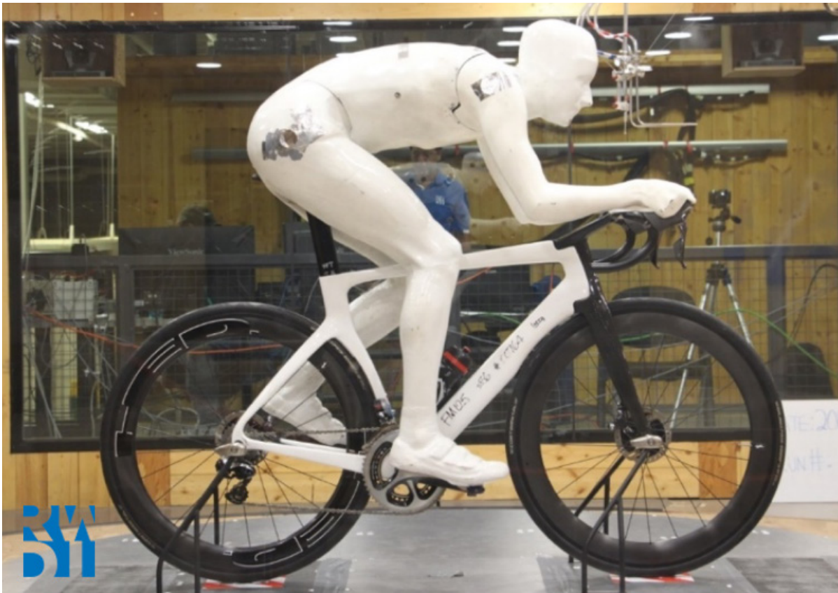
Figure 5. Wind tunnel test setup with S5 and anthropomorphic rider model.
