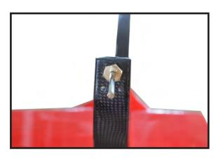
Align the wheel pant slot over the axle bolt as shown. Slide the wheel pant slot over the flat sides of the axle bolt and align blind nuts in wheel pants with mounting holes in landing gear. When all bolt holes are aligned tighten axle in place.
