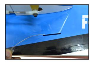
9) Thread cable through brass swage tube.
