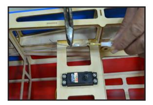
14) Attach ball links to the rudder servo arm and then attach the servo arm to the rudder servo as shown.
