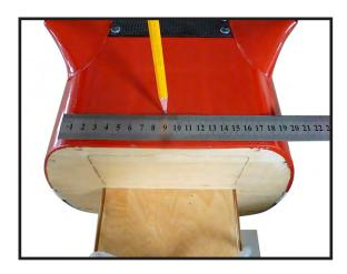
4) Aligning center lines of template and fuse. Tape the template to the bottom of the fuse with the back edge of the template flush against the aft edge of the recessed cowl mounting ring.
