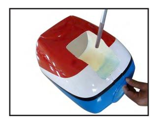
12) Install the cowl and check that everything fits correctly and does not come in contact with the cowl. If needed enlarge the cutouts and test fit again until everything fits correctly.
