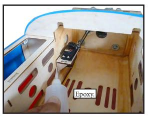
6) Reinstall the servo horn by sliding the connector over the pushrod wire. Center the throttle stick and trim and install the servo horn perpendicular to the servo center line.
