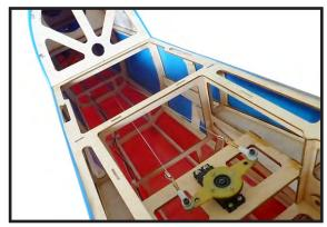
**NOTE**: <u>Cable is installed crossed "X"</u>, not parallel.
