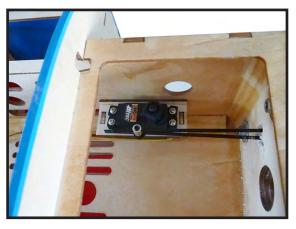
7) Move the throttle stick to the closed position and move the carburetor to closed. Use a 2.5mm hex wrench to tighten the screw that secures the throttle pushrod wire. Make sure to use threadlock on the screw so it does not vibrate loose.
