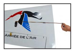
3) Attach the extension to the servo lead and secure with Safety Clip, safety wire, tape or other method. Ensure the plugs will not come apart from vibration or light tension.
