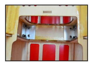
Install gear cover into landing gear.
