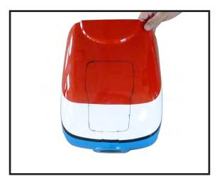
11) Remove the template and use a rotary cutting tool and sanding drum to cut out the openings in the cowl.
