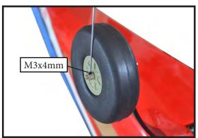
Use blue Loctite on the bolts before final tightening.
