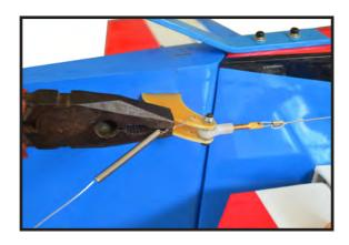
Do same for attachment the steering spring to the rudder tiller.
