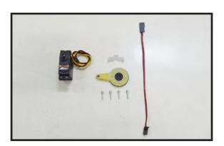
2) Layout the servo on the wing to test fit the installation and ensure servo lead is the correct length.
