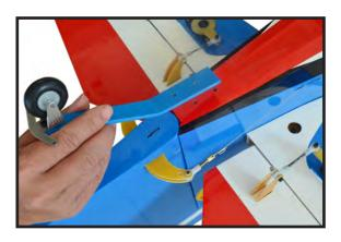
Place a drop of Blue Loctite on tail wheel strut mounting screws.
