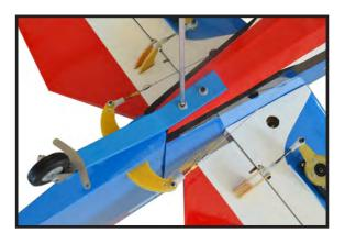
Attach the steering spring to the rudder control horn.
