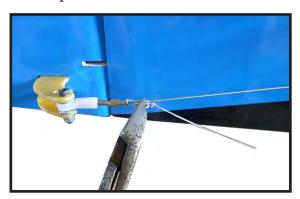
6) Cut off excess cable as shown.
