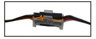
4) Fasten the pull string from the servo hole to the male plug of the servo extension.
