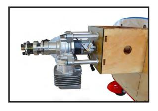
Using mounting bolts and washers mount engine to firewall.
