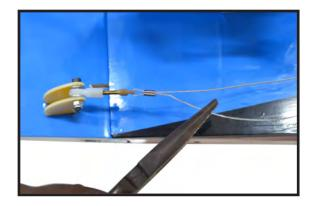
5) Crimp the brass tube with a crimping tool or pliers.
