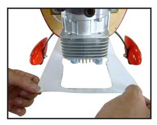
9) Fit template flush with rear of cowl and align center marks of template and cowl. Tape template to the bottom of cowl. Use a felt tip marker to transfer the template cutout pattern to the cowl and mark cut location.
