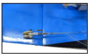
4) Loop the cable back through the brass swage tube and tighten the second loop through the brass swage tube as shown.
