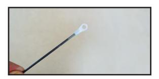
3) Attach throttle pushrod to the carburetor throttle arm with the ball link.
