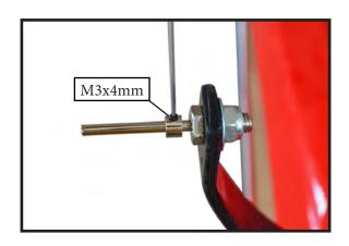
Install the wheel and outer wheel collar. Use blue Loctite on the wheel collar set screw before final tightening
