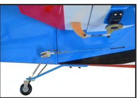
INSTALLING THE MAIN LANDING GEAR TO FUSELAGE.
