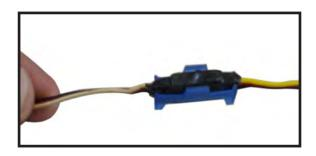
3) Feed servo extension through the elevator servo mounting hole.
