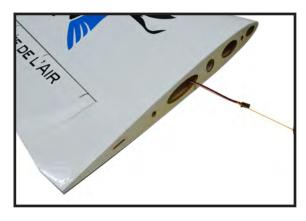
5) Install servo in servo well with the output arm toward the leading edge of the wing. Mark and drill location of servo mounting holes.
