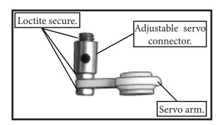
5) Install throttle servo into servo mounting tray.
