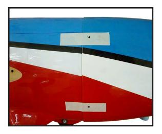
14) Mark by using a drill to drill the holes for the cowl mounting screws. Then, take cowling out of and drill on it. Make sure the cowl position is correct before drilling each hole.
