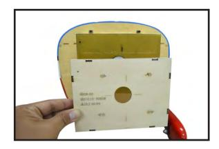
Use a 1/4 bit to drill the engine mounting holes
