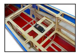
8) Feed one rudder cable through the pre installed cable exit tube in the rear of the fuse toward the front of the fuse. Repeat for other side.
