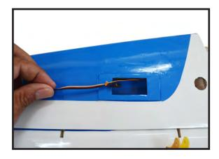
4) Mark and drill location of servo mounting holes.
