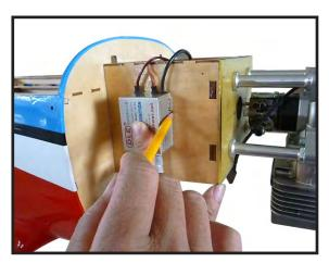
2) Use a 1/8" bit to drill the ignition module mounting holes.
