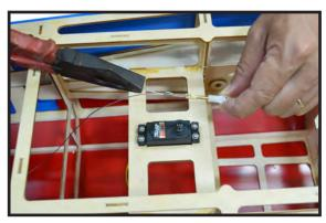
12) Crimp the brass swage tube with a crimping tool or pliers.
