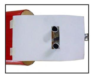
6) Trace around the head of the engine being careful to keep the template in the same location.
