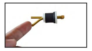
1) Install the fuel tubing and clunk. Secure the fuel tubing with nylon ties to the pick-up tube and clunk.
