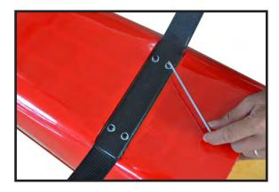
Use lock nut to secure landing gear tighen into fuselage.
