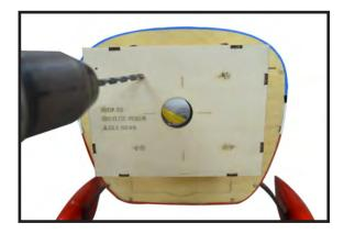
Remove mounting template from firewall. Firewall shown with mounting holes drilled ready for engine mounting.
