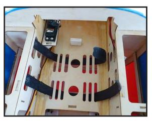
Slide the fuel tank into the fuselage. Use the T-fiting from the fuel dot to connect lines from the clunk to the carburetor. Secure all connections using tie wraps.
