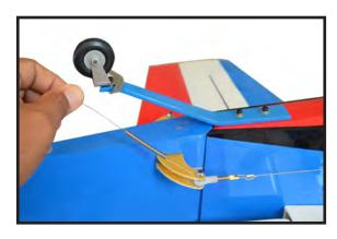
Use pliers to twist spring end closed around rudder control horn.
