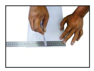
3) Measure and mark the center of the bottom of the fuselage as shown. Mount cowling to fuse and transfer center line on fuse to bottom of cowl.
