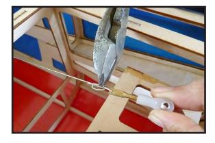
13) Cut off excess cable as shown.
