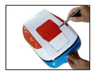
10) The cowl should be marked as shown. Be sure to mark all of the lines clearly and carefully to aid in cutting.
