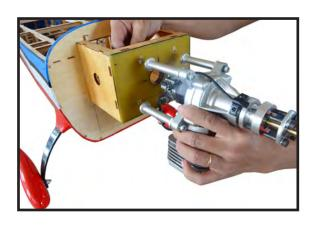
Tighten mounting bolts and secure engine to firewall.
