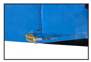
7) Mark and use a 1/16 bit to drill the rudder servo.
