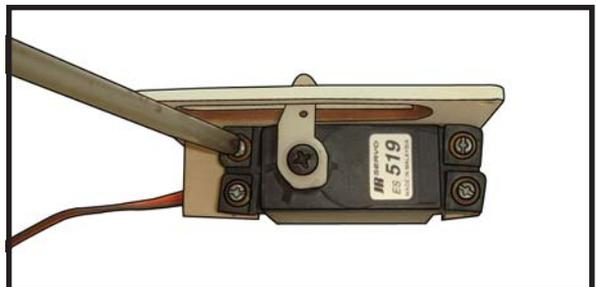
7) Apply 1-2 drops of thin C/A to each of the mounting tabs. Allow the C/A to cure without using accelerator.
