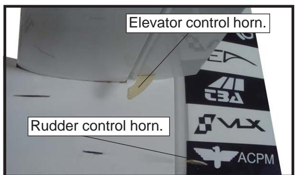
□ 3) Thread one clevis and M3 lock nut on to each elevator control rod. Thread the horns on until they are flush with the ends of the control rods.
