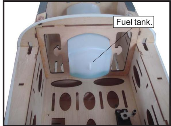
□ 8) Use plywood template to hold in place the fuel tank with C/A glue to secure the fuel tank inside the fuselage.
