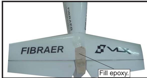
3) Slide the vertical stabilizer back in place. Using a triangle, check to ensure that the vertical stabilizer is aligned 90° to the horizontal stabilizer.
