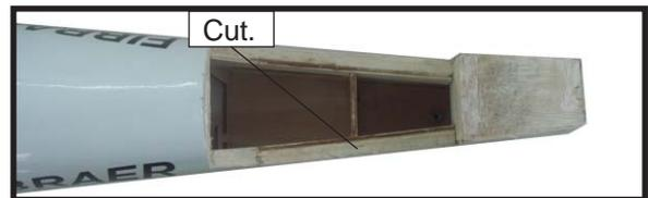
□ 3) Slide the stabilizer into place in the pre-cut slot in the rear of the fuselage. The stabilizer should be pushed firmly against the front of the slot.
