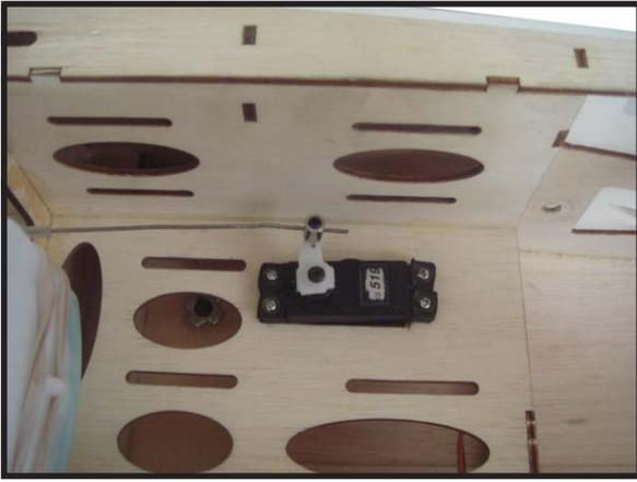
9) Move the throttle stick to the closed position and move the carburetor to closed. Use a 2.5mm hex wrench to tighten the screw that secures the throttle pushrod wire. Make sure to use threadlock on the screw so it does not vibrate loose.
