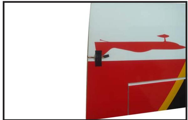
9) Set the aileron hatch in place and use a Phillips screw driver to install it with four wood screws.
