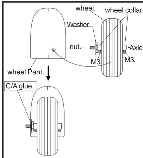
□ 5) Place the wheel assembly in the wheel pants. The threaded portion of the axle will fit the notch of the wheel pants as shown.
