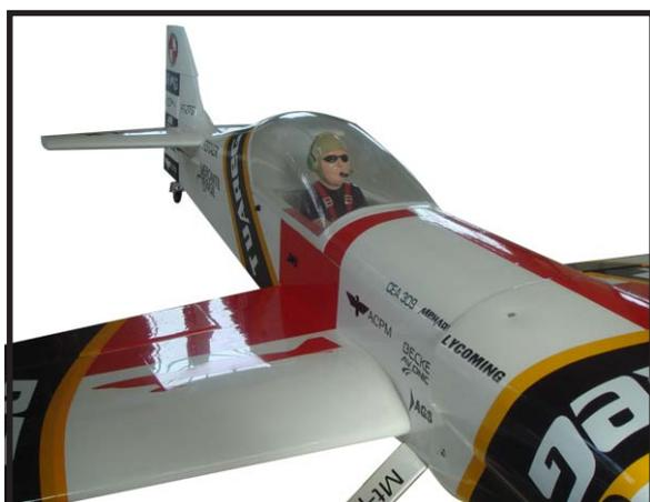
With the wing attached to the fuselage, all parts of the model installed ( ready to fly), and empty fuel tanks, hold the model at the marked balance point with the stabilizer level.
